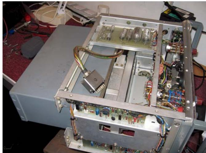
Once removed and the cover slid off the RF unit, it became apparent that the circuit I had did match some of the filter boards. All of the voltages and control lines into the RF unit go through two filter sections. The filters are wound on plastic formers and housed in ferrite pots. I found no less than 12 of these filters to be open circuit.
