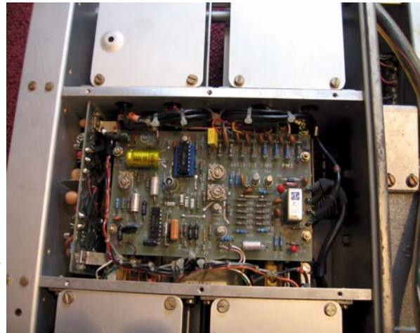
The level of the raw oscillator was checked and this was found to be OK. I could not find any reason for the carrier meter to be showing a low level. The meter sits at the centre of a bridge circuit formed by two resistors and two diodes. This all check out OK.
