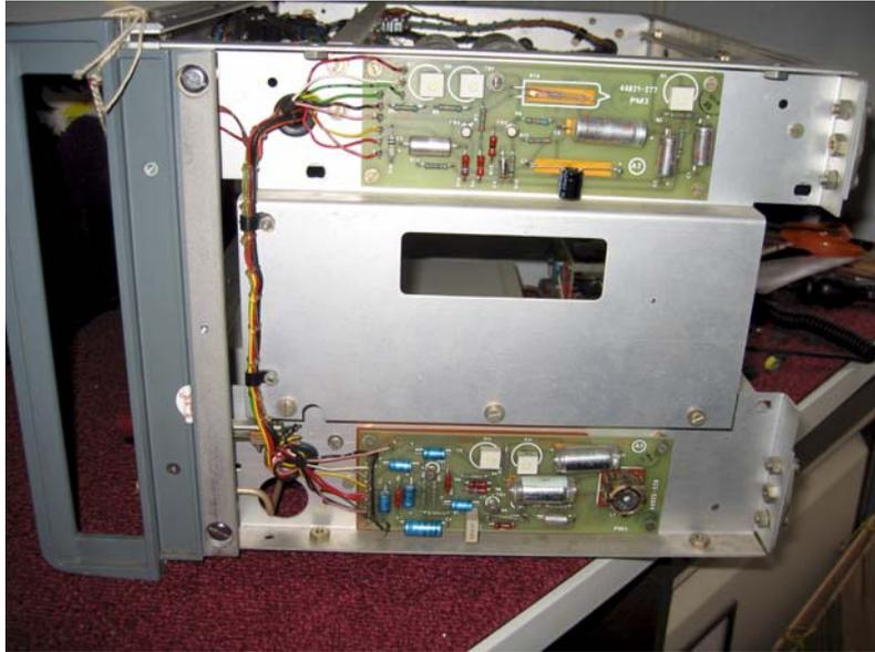
There was still no RF output and no RF indication on the Carrier meter. This left no alternative but to remove the RF unit for examination and repair. The design of the unit makes this a simple task. Removing four screws in the side of the unit allows the whole unit including scale and knobs to be drawn out through the back of the instrument. The module plugs into the carcase via a multi-way plug and socket. Here you can see the RF unit half way out.
