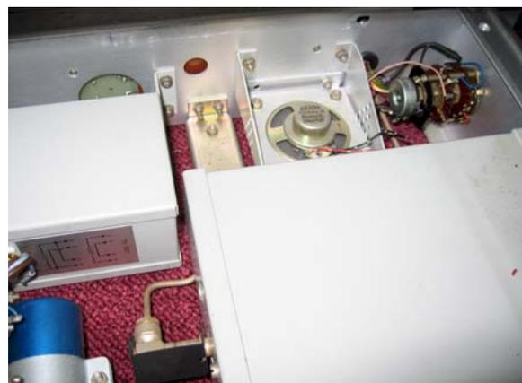
Finally the RF output level was checked. With the RF attenuator switched to zero, the output level should be 1v into 50 ohms. This is normally done with an RF voltmeter, but I used a spectrum analyser. The 1v output should coincide with the Carrier level meter red calibration mark. All OK.
