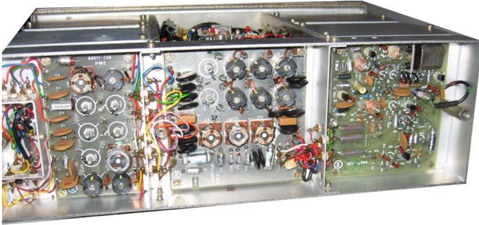
Here is a view of the two filter sections, extreme left and centre. To the right is the calibrator oscillator. In this picture you can see where I have removed 8 of the cores. To fit the new components I lifted the PCB and removed the metal studs which can be seen in the photo. This provided the extra space needed to fit the new inductors which were soldered to the original tags.
