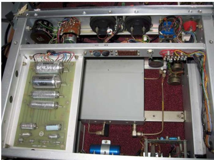
In this photo can be seen bottom left the suflex capacitors which are switched into the Wien oscillator to produce the audio for modulation.
