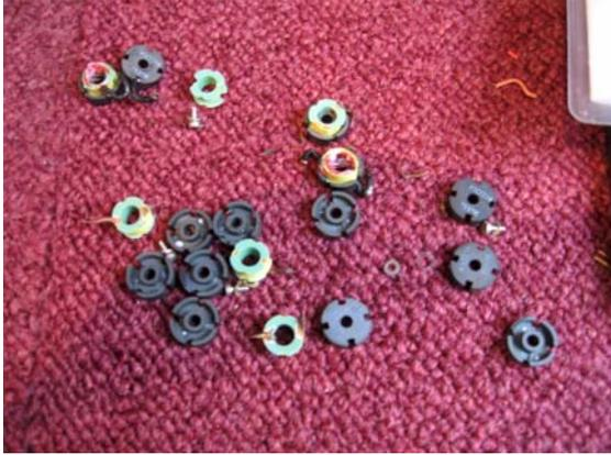
The filters which were removed after being tested with an ohm-meter. Most read High Ks of resistance and should have been in the low 10s of ohms.
